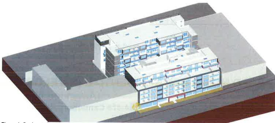
Figure 1: Geolocated model of JRPP scheme in SketchUp: view from the sun at 12 noon
